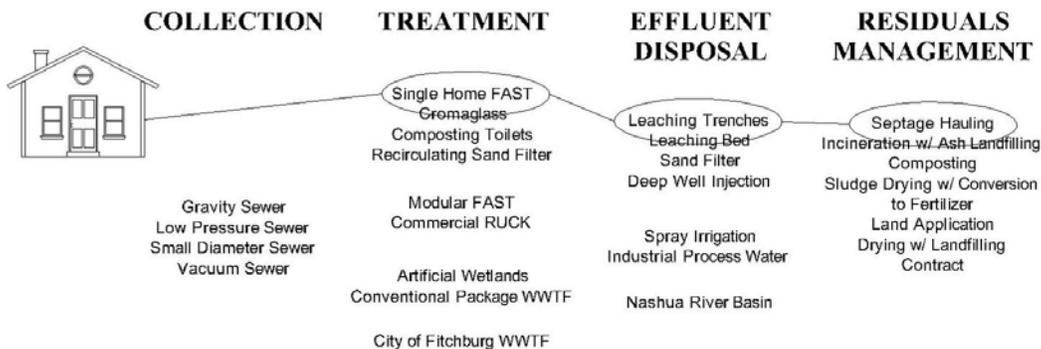
The cost to install a new conventional on-site system (Title 5 subsurface disposal system) generally ranges between \$10,000 and \$25,000, based on site conditions (2006 dollars). The only regular maintenance requirement is the cost to pump out the septic tank, which is typically \$150 to \$250, and should be done every three to five years.
