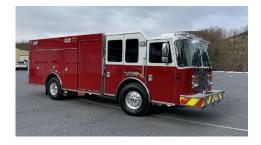
Engine 2 – (2001 Class A Pumper) KME. This vehicle has a 1,500gpm pump with 2,500 gallons of water. This vehicle is also equipped with a Class A foam system which increases the vehicles fire suppression ability. This vehicle is a dual role vehicle able to perform as an attack pumper or a tanker for incidents in areas of town with no hydrants. This vehicle was refurbished in 2018 and is in good shape.
